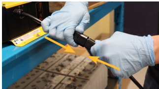
Figure 3: Reconnect AC power to the charger.
