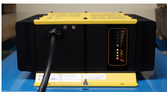
Figure 4: Charger LED indicator self-test.
