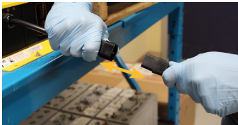
Figure 1: Disconnect AC power.
